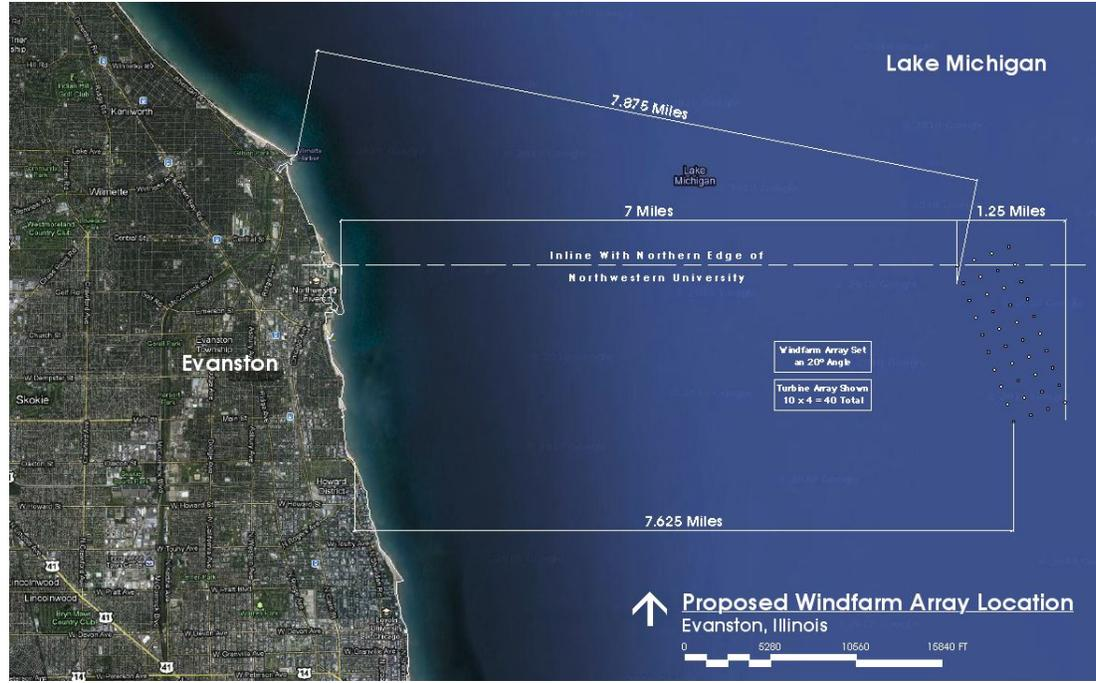
The working concept places the turbines approximately seven miles off the Evanston shore stretching between Northwestern's northern boundary to the southern edge of Daves Park. The current notion for the layout of the wind farm is to have the turbines arrayed in rows slightly angled from the northwest to the southeast. This layout will limit the visual impact of the turbines both to the north and south of the site.
