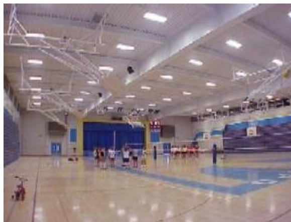
In this gym, if one lamp fails in a fixture, other lamps in the same fixture will continue to produce light. Photo courtesy of Sacramento Municipal Utility District.
